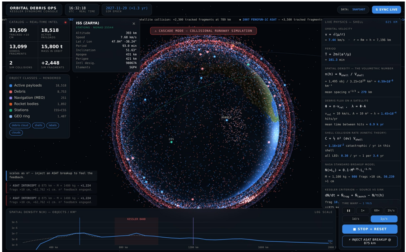
Figure B-2 — Cascade mode, +1.3 simulated years after two ASAT injections at 875 km: tracked objects 29,163 → 33,509, +2,448 fragments >10 cm, all-LEO collision rate 0.18 → 0.30/yr, and the live density curve (solid) lifted above the t_0 baseline (dashed) through the 300–900 km band.
